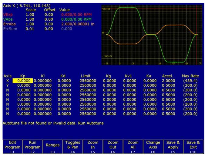
This error is due to a delay time mismatch. Centroid autotune has corrected the delay to the best of its ability, but the smallest correction it can make is 250us. A residual delay mismatch may remain that is between 0 and 250us.
