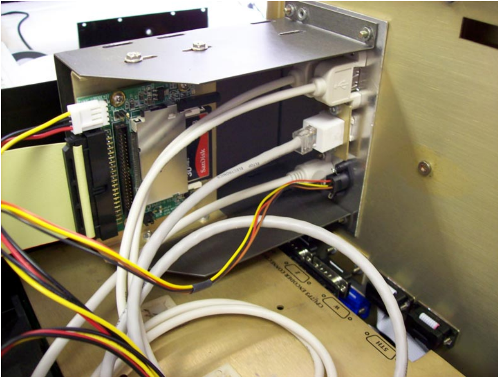
Picture 2: This is how the I/O panel and floppy drive bay w/ SSHD should be mounted.
