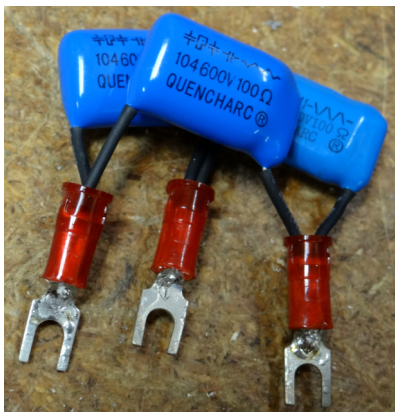
Picture 2: Quencharc assembly for 3-Phase motor (Centroid PN: 12610)
