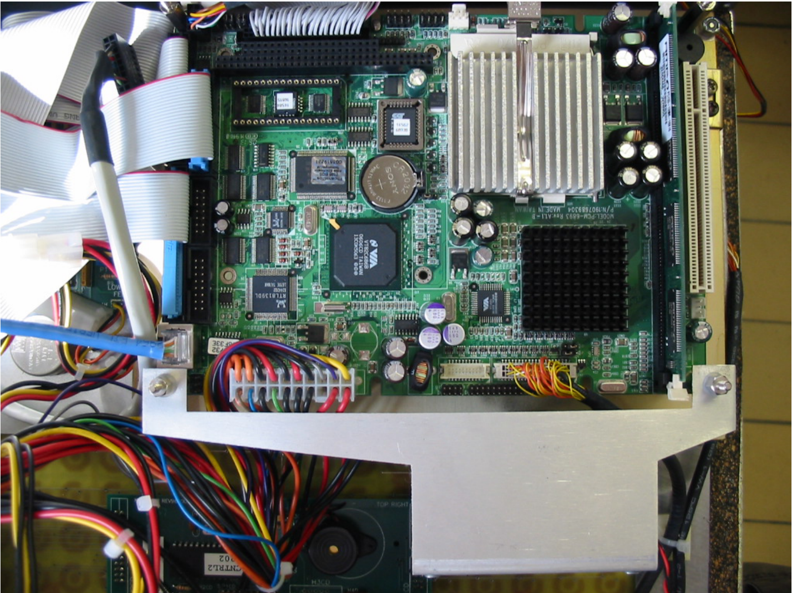
Picture 3. Aeon motherboard installed in an M400
