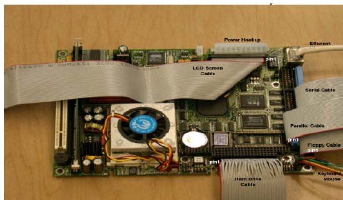
Picture 1: Aaeon with cables inserted correctly:
