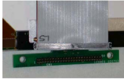
Picture 4: Aaeon motherboard LCD Descrambler card:
