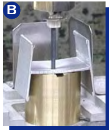
A-B-C: Even after being pressed into a sheet of metal, the SiNi ignitor performed perfectly.
